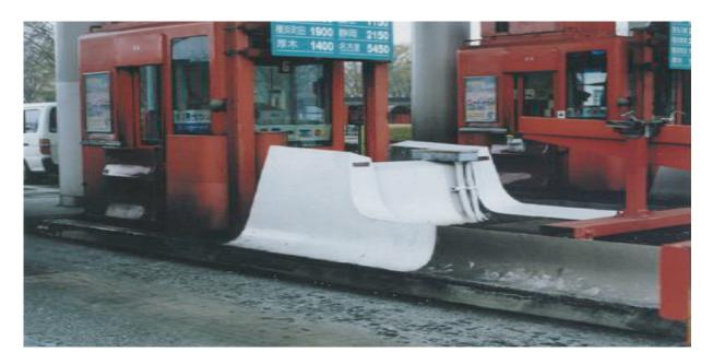
This photo shows a white concrete panel exposed to six months of highway grime. The white squares had been coated with our TPXsol phocatalyst self cleaning coating.
