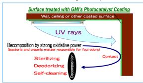
**STERLIZATION** — Titanium dioxide has strong oxidation affects to single-celled organism that includes all bacteria and fungus. The very strong oxidizing power of Titanium Dioxide can destroy bacteria's cell membrane, causing leakage of the cytoplasm, which inhibits bacteria's activity and ultimately results in the death and decomposition of bacteria. Generally speaking, disinfections by titanium dioxide is three times stronger than chlorination, and 1.5 times stronger than ozonation.
