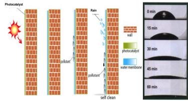
**The** hydrophilic nature of titanium dioxide, coupled with the gravity, will enable the dust particles to be swept away following the water stream, thus making the product self-cleaning.
