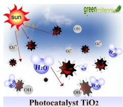
**When** photocatalyst is exposed to light in the presence of water vapor, two highly reactive substances are formed: hydroxyl radicals [OH] and a superoxide anion  $[O_2^{-1}]$ . It allows the oxidation of airborne VOCs convert into carbon dioxide and water at room temperature with UV or near-UV light source. It does not need a special energy and use only clean energy in ordinary life.
